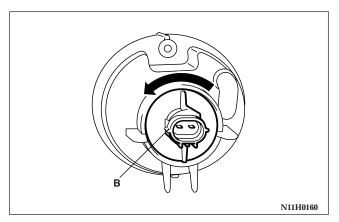
3. Remove the entire socket and bulb assembly (B) by turning it counterclockwise.
